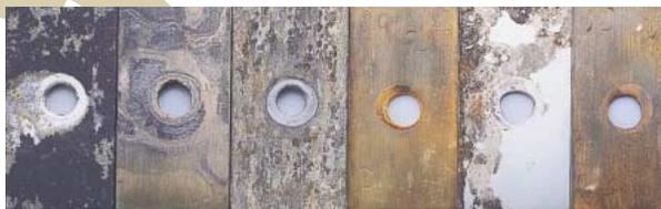
Cast Aluminum Cast Iron Solder Brass Steel Copper
